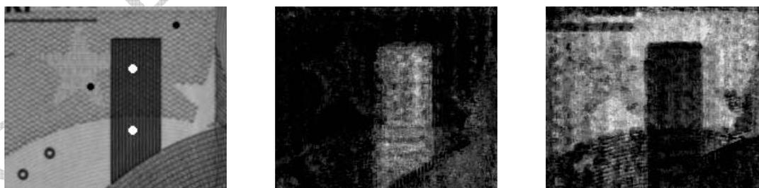
Figure 9: Closeup of experiment with two reference points. The left image shows two reference points in the intaglio print area (white) and two reference points in the offset print area (black). The two other images visualize the degree to which a pixel belongs to the intaglio print area (middle) and the offset print area (right)
